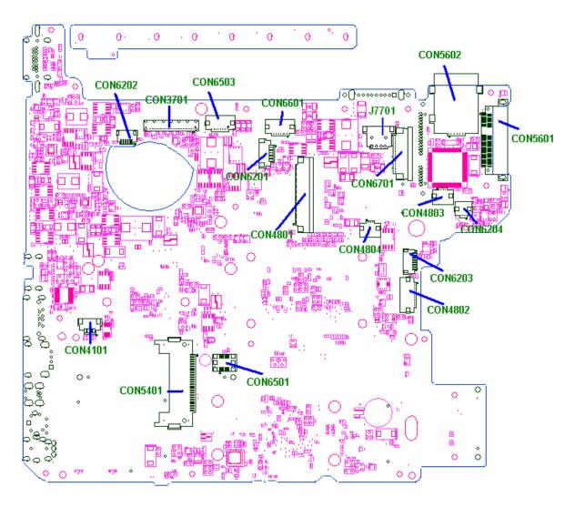
Figure B-1 Main board layout (front)
